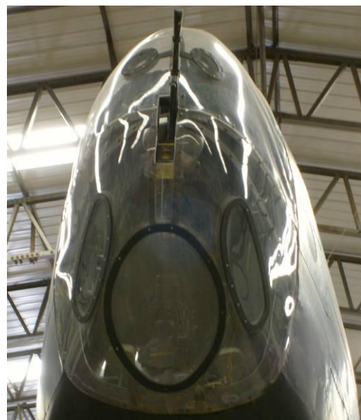
Figure 2 Bomb aimer's position in the nose of a Halifax MkIII
